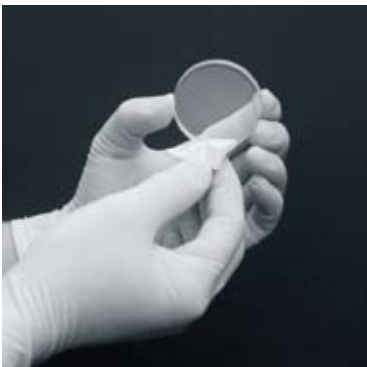
Figure 2. Blotting the lower edge of device without contacting the coated surface.
