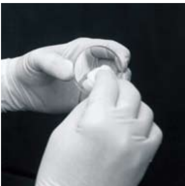
Figure 3. An alcohol-saturated cotton ball can be used to gently pat the surface.
