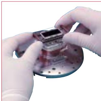
Figure 4. XP detector being assembled at Princeton Instruments' state-of-the-art manufacturing facility.
