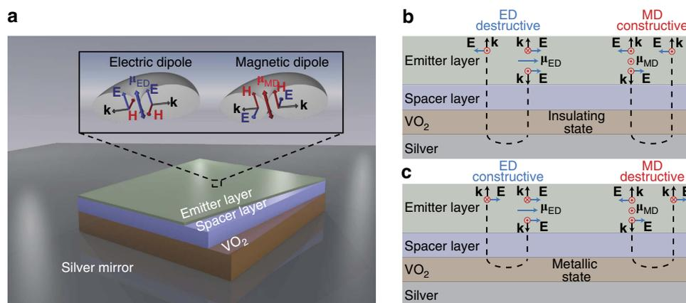
**Figure 1 | Sketch of the sample and illustration of LDOS modulation.** (a) Sketch of the sample. Inset shows the polarization symmetries of ED and MD radiation. (b,c) illustrate the interference of ED and MD emission processes when the VO<sub>2</sub> layer is in the insulating and metallic phases, respectively.
