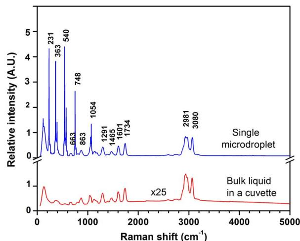
**Fig. 2.** Raman scattering spectra of diethyl phthalate from a single laser-trapped 21  $\mu\text{m}$  microdroplet in the air (blue trace) or bulk liquid (red trace) in a cuvette. The recording integration time for each spectrum is 2 s.
