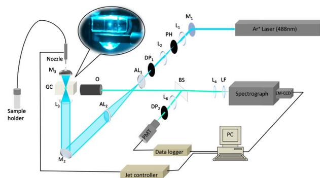
**Fig. 1.** Schematic of the experimental setup for a laser-trapping single-particle Raman spectroscopic system.  $M_1$ : mirror,  $L_1$ : lens, PH: pin hole,  $DP_1$ : diaphragm,  $AL_1$ : axicon lens, O: objective lens, GC: glass cell, BS: beam splitter, LF: long-pass filter, EM-CCD: electron multiplying charge coupled device, PMT: photomultiplier tube.
