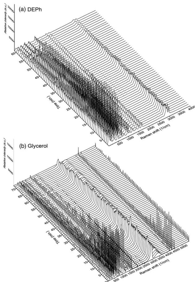
**Fig. 3.** Time evolution of the Raman spectrum of an optically trapped (a) DEPh and (b) glycerol microdroplet. Spectra were continuously recorded for about an hour at a 1 min interval with a 2 s integration time as the particle size changed from about 20  $\mu\text{m}$  to about 17  $\mu\text{m}$  in diameter.
