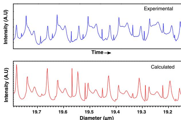
**Fig. 5.** Comparison between the experimental and calculated resonance spectra of the elastic scattering intensity at  $90^\circ$  from a laser-trapped diethyl phthalate microdroplet from  $19.8\ \mu\text{m}$  to  $19.15\ \mu\text{m}$  in diameter.
