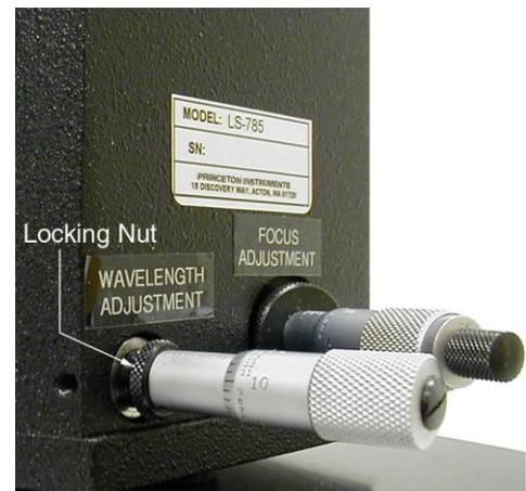
Figure 2-4. Wavelength Adjustment Micrometer
