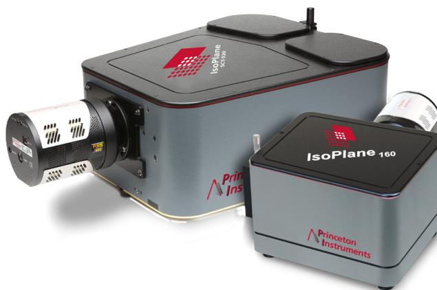
Another imaging spectrograph available from Princeton Instruments, the IsoPlane-320, utilizes a unique optical design that completely eliminates astigmatism across the entire focal plane to deliver superior multichannel capabilities. This patented, multi-award-winning instrument boasts fast f/4.6 optics and exceptional image quality, ensuring maximum throughput and signal-to-noise performance.
