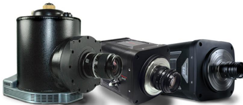
First and foremost, either maintenance-free thermoelectric cooling or liquid nitrogen can be employed to chill the NIRvana’s two-dimensional 640 x 512 InGaAs FPA detector down as low as  $-85^{\circ}\text{C}$  or  $-190^{\circ}\text{C}$ , respectively. A proprietary cold shield design and vacuum technology facilitates the lowest possible dark noise, which helps increase sensitivity as well as preserve signal-to-noise ratio (SNR) for long exposure times.
