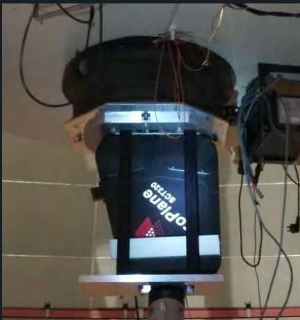
PIXIS camera and IsoPlane 320 spectrometer used for spectroscopic detection of space debris test at SHAO 60 cm telescope. Photo courtesy of Prof. Zhenghong Tang, Shanghai Astronomical Observatory, Chinese Academy of Sciences.
