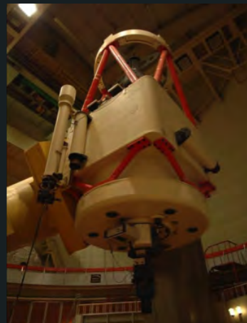
A cryogenically cooled Princeton Instruments CCD camera installed on the 2.16 meter reflector at Xinglong Observatory, NAOC.
