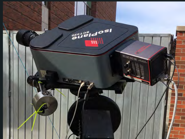
BLAZE camera and IsoPlane 320 spectrometer used to observe 8-21-17 solar eclipse from Willamette University (Salem, Oregon). Photo courtesy of Ronald Dantowitz, Clay Center Observatory Director, Dexter Southfield School (Brookline, Massachusetts).
