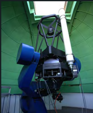
A cryogenically cooled Princeton Instruments CCD camera installed on the 80 cm reflector at Xinglong Observatory in China.
