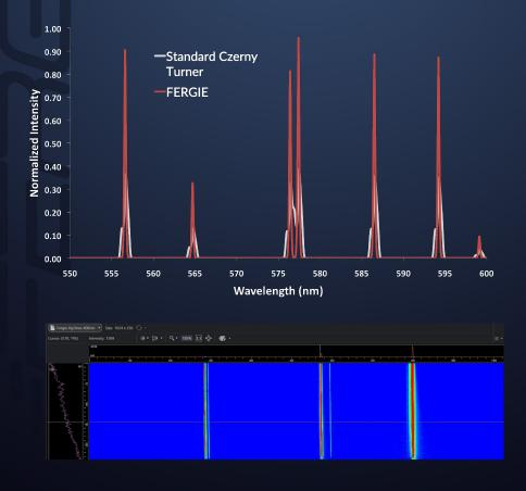
(Top) Comparison of spectral data from the optical design of a standard 300 mm Czerny Turner spectrometer and FERGIE.
