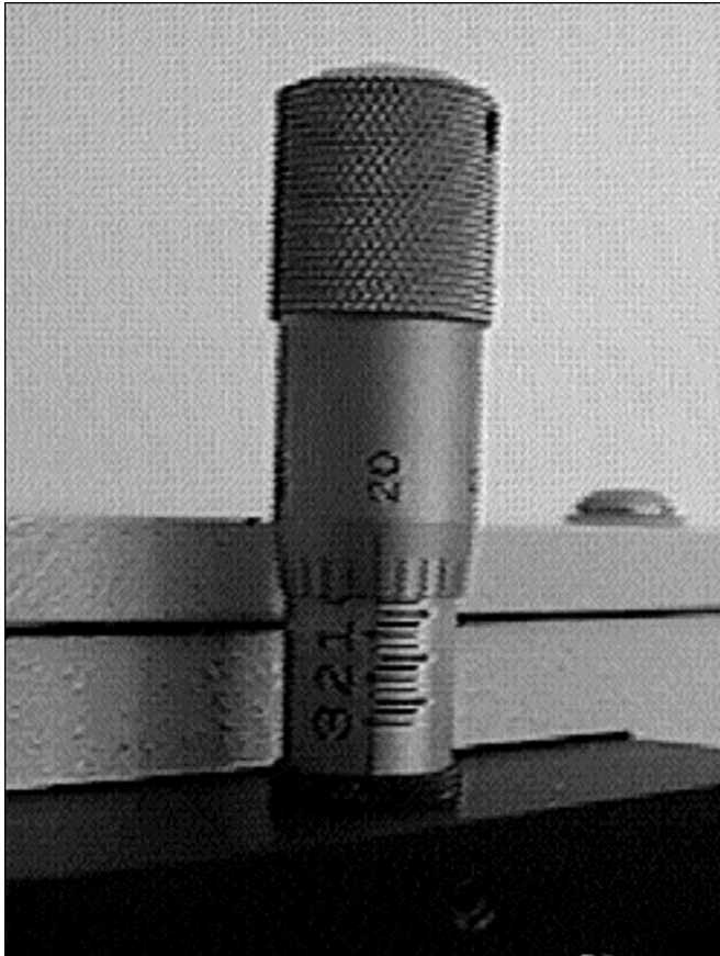
Slit Width Setting: 200 Micrometers (0.200mm)
