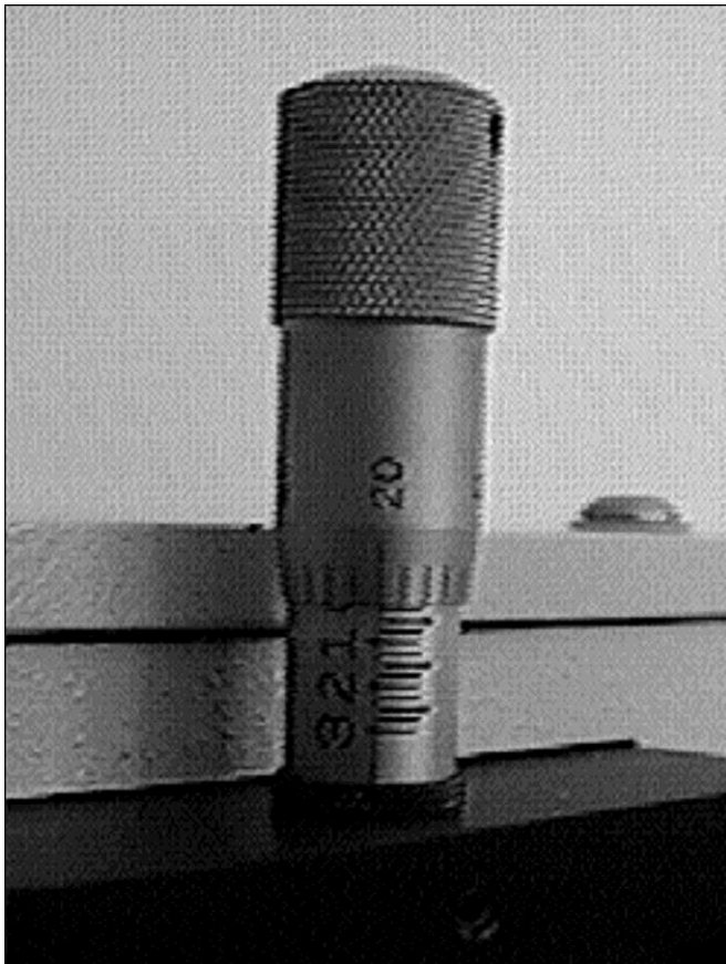
Slit Width Setting: 200 Micrometers (0.200mm)
