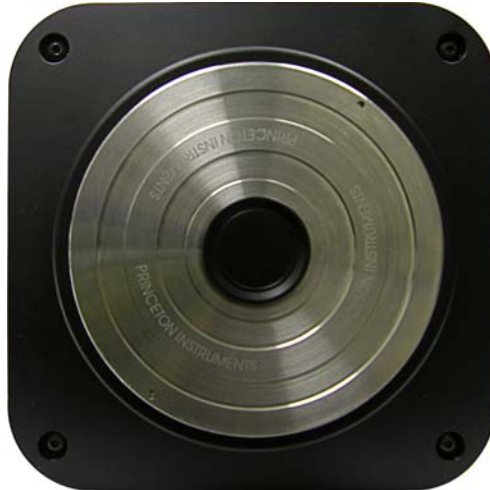
Figure D-2: Remove Screws Securing the Camera's Front End
