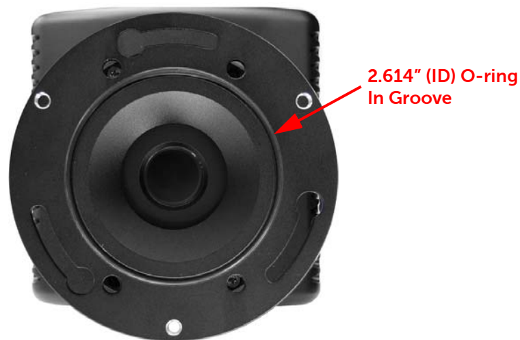
Figure G-5: Positioning the 2.614" (ID) O-ring
