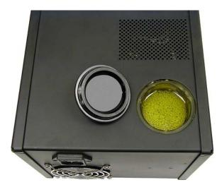
If additional coolant is required, fill with a 50:50 mixture of water and ethylene glycol.
