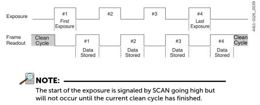
The configuration of clean cycles is performed on the **Hardware Setup**  $\triangleright$  **Cleans/Skips** tab {via the **Sensor Cleaning** pane accessed on the **Sensor** expander}. When you set up the camera for the first time, default values are automatically inserted into these fields. These will give the best results for most applications. Even so it is a good idea to know what these entries mean with regard to cleaning.
