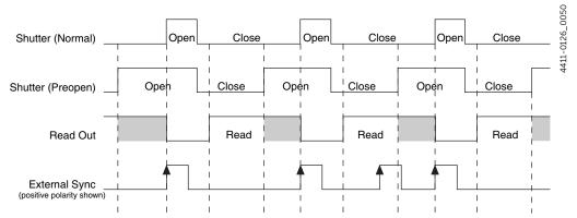
Figure 6-5: Timing Diagram: WinX/32 Continuous Cleans
