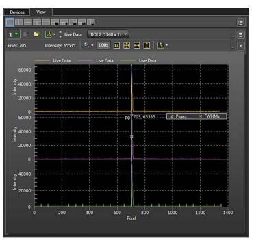
When aligning accessories (e.g., fibers, lenses, optical fiber adapters,) first align the spectrograph to the slit. Then align the accessory without disturbing the camera position. The procedure is identical to that used to focus a spectrograph (i.e., focus and align while watching a live image).
