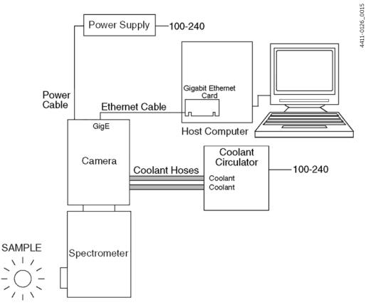
Figure 3-4: Block Diagram: Typical Spectroscopy Experiment with Air/Liquid-Cooled ProEM
