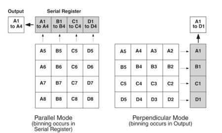
You can easily switch between these orientations by rotating the camera 90° and changing the binning parameters in the application software.
