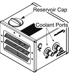
**4.** It is recommended that hoses be secured to the camera hose barbs with the clamp supplied.
