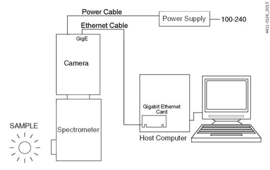
Figure 3-2: Block Diagram: Typical Spectroscopy Experiment with Air-Cooled ProEM
