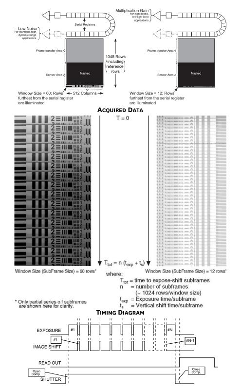
Figure 6-12: Kinetics Mode: Partial CCD Illumination, ProEM:512B
