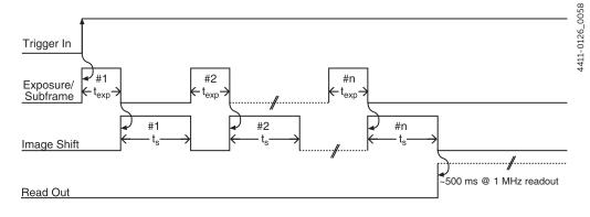
Figure 6-13: Timing Diagram: Kinetics Mode, Single Trigger {Readout Per Trigger}
