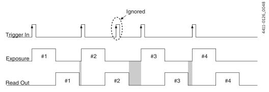
For a sequence of one frame, bulb mode and trigger-first mode are the same. The
