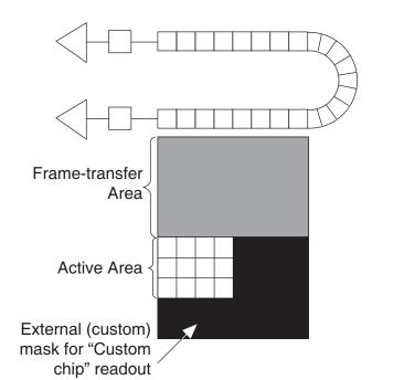
Figure 6-20: Functional Block Diagram: CCD Array
