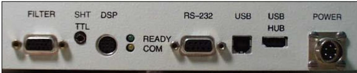
Figure 19. Cable Connections (Back Panel)
