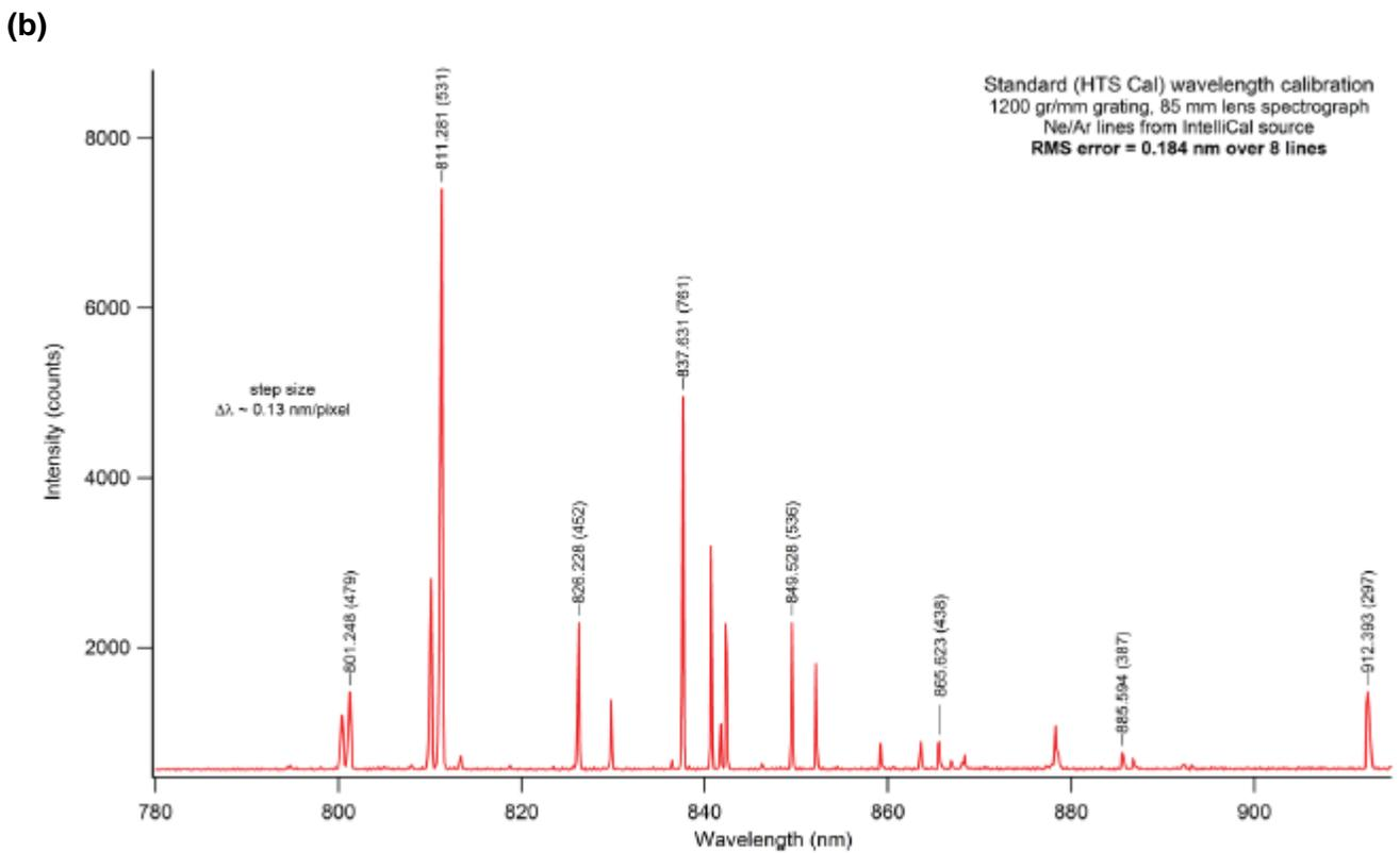
**Figure 4.** Calibration error for an Acton Series LS785 spectrograph from Princeton Instruments utilizing (a) IntelliCal and (b) standard routines.
