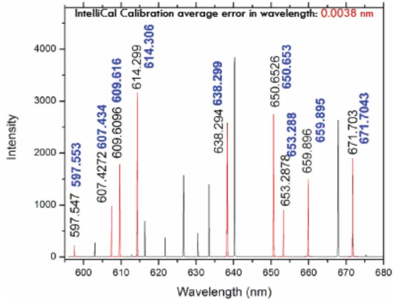
Post-refinement capabilities are impressive as well. These include simulating how any emission spectrum will appear at the detector for an arbitrary grating position, seamless combination with a pattern recognition algorithm, and searching all possible grating angles so as to fully determine the state of the instrument.
