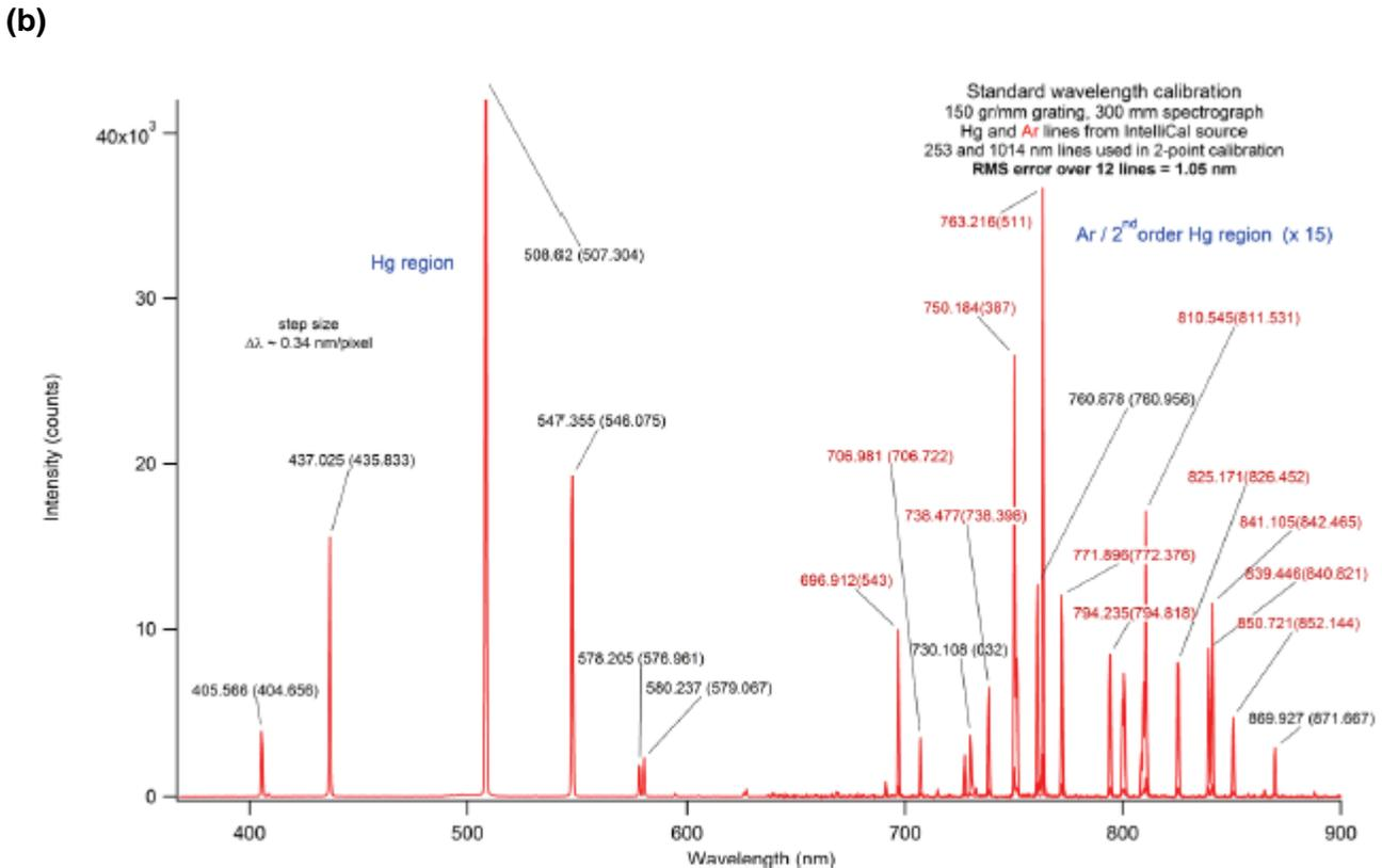
**Figure 3.** Calibration error for an Acton Series SP2300 spectrograph from Princeton Instruments utilizing (a) IntelliCal and (b) standard routines. The relatively high RMS calibration error is due to the low dispersion of the grating used; much greater accuracies can be obtained with high-groove-density gratings.
