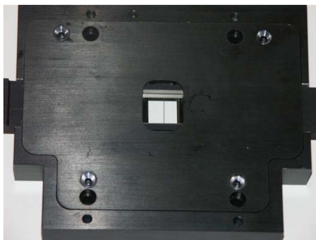
Figure 28. Intermediate Slit with 150 \mu\text{m} Laser Stop
