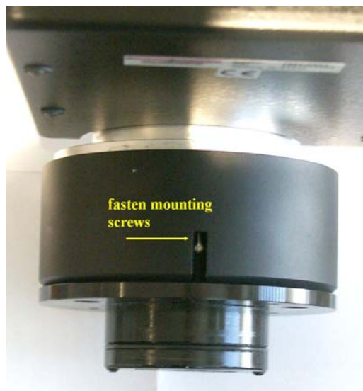
Figure 100. Assembled Mount on the Nose of an LN-cooled Diode Array Detector
