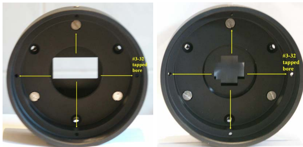
Figure 99. Mounting Spectrograph Flange to CCD-mount without Shutter. Left: with Baffle from 500 mm Spectrograph, right with Baffle from 750 mm Spectrograph
