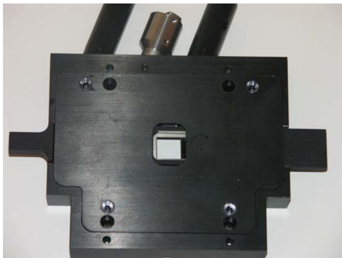
Figure 29. Intermediate Slit with Open Laser Stop
