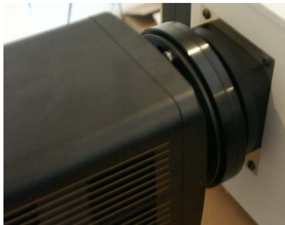
Figure 94. Mounted Peltier-cooled Diode Array Detector
