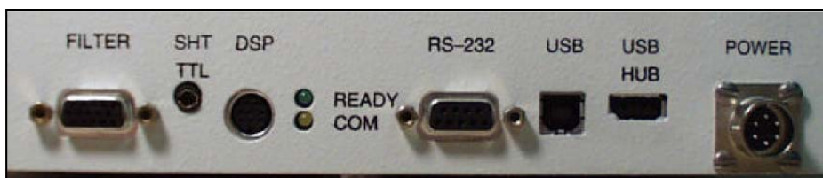
Figure 7. Spectrograph Cable Connections
