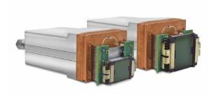
The back-illuminated CCDs (large 2k x 2k or 4k x 4k formats) utilized by the PI-MTE3 platform offer >95% peak quantum efficiency. Efficient liquid cooling results in low dark current, facilitating long integration times.
