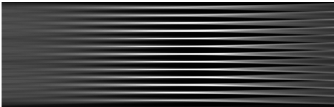
Figure 4: Multitrack spectroscopy on a Czerny-Turner spectrograph. The signal traces are broadened vertically by astigmatism with increasing severity towards the edges of the focal plane.
