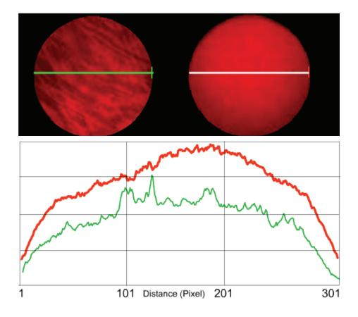
Reduced etaloning: CCD PIXIS etaloning-Comparison of Standard Back-Illuminated CCD vs. eXcelon BI CCD
