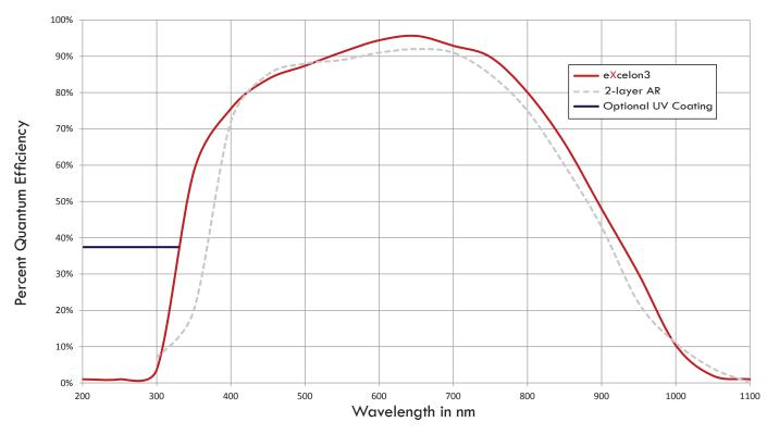
NOTE: Graph shows typical Quantum Efficiency (QE) data measured at + 25° C. Quantum Efficiency is a function of temperature and actual results will depend upon CCD temperature.
