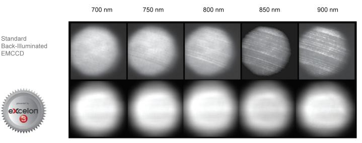
Data taken with white light source through a monochromator comparing fringe supression of eXcelon vs. conventional back-illuminated EMCCDs.
