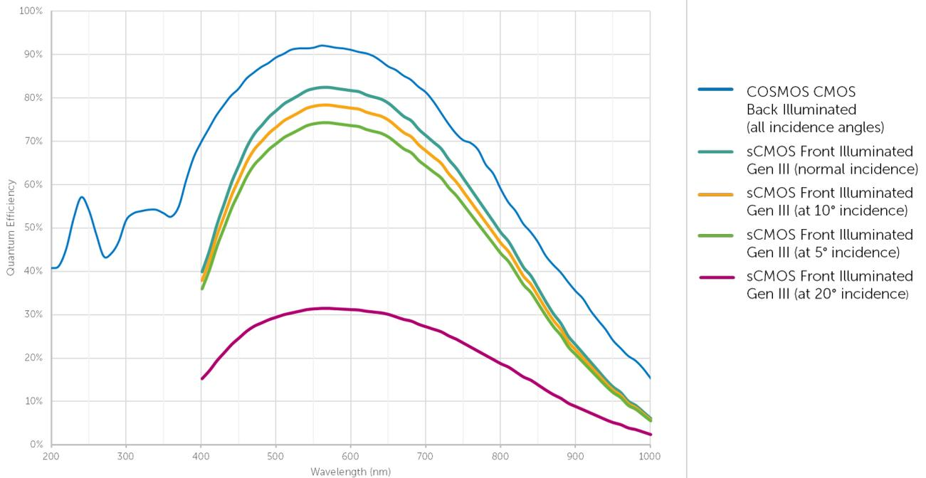
**Figure 3:** Quantum efficiency (QE) of the COSMOS with respect to wavelength, showing 90% peak quantum efficiency, and a typical front illuminated sCMOS Gen III sensor at normal incidence, 10° incidence, 5° incidence and 20° incidence showing how QE drastically decreases in front illuminated with angle of incidence.
