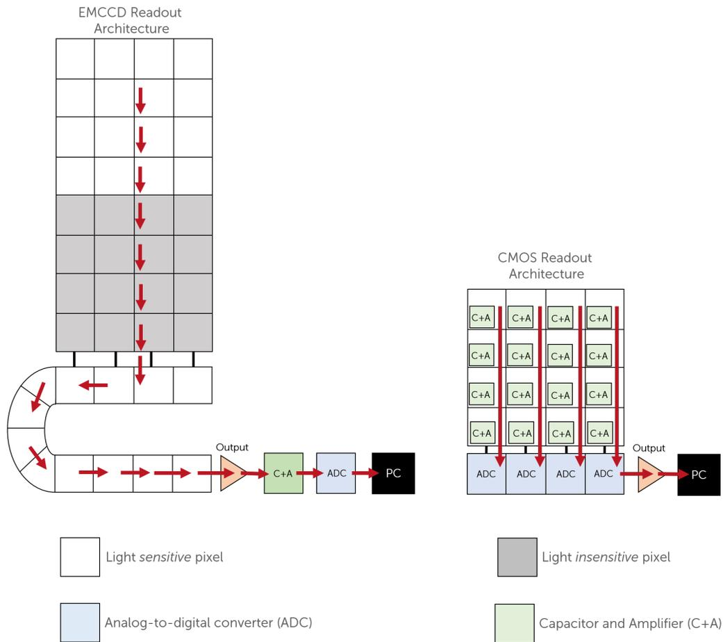
**Figure 4:** Sensor readout architecture of a typical EMCCD and a typical CMOS. The individual electronics on each pixel, and the ADC for each column greatly increases the speed at which acquired data can be processed.
