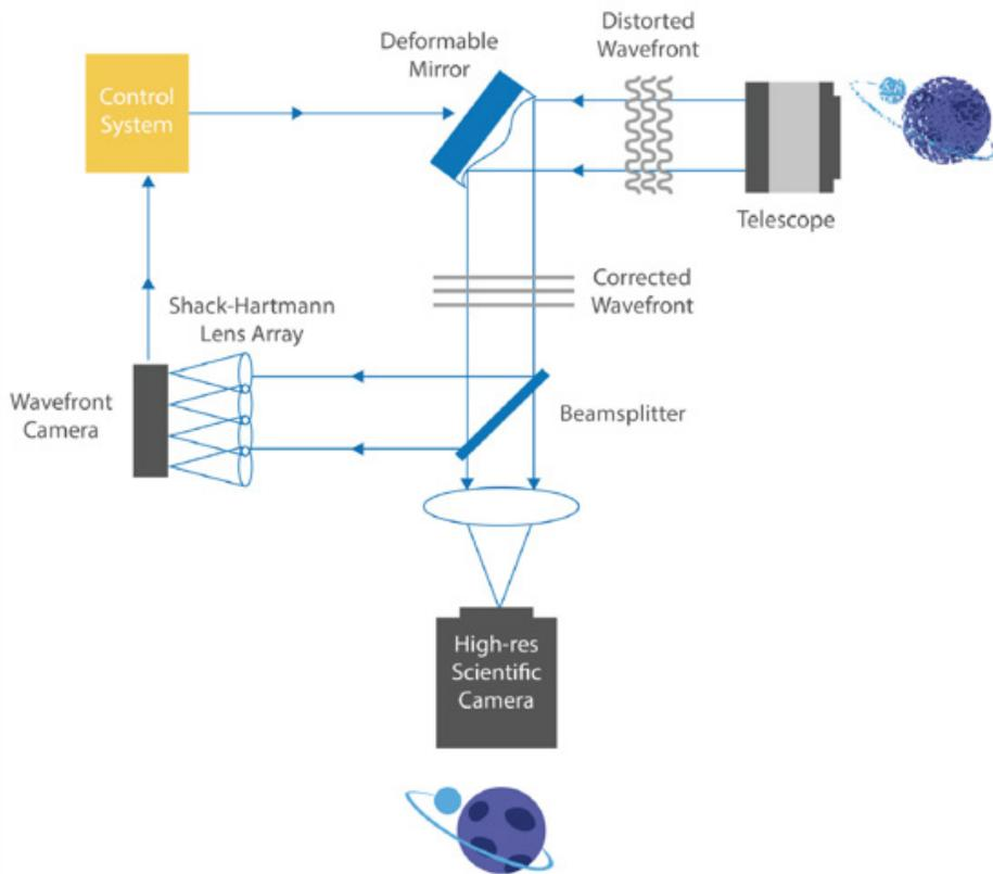
**Figure 1:** Schematic of an adaptive optics system in which a distorted wavefront is measured by a wavefront camera, which feeds the level of distortion into a control system. This control system counteracts the distortion via a deformable mirror which corrects the wavefront to produce a diffraction limited image.
