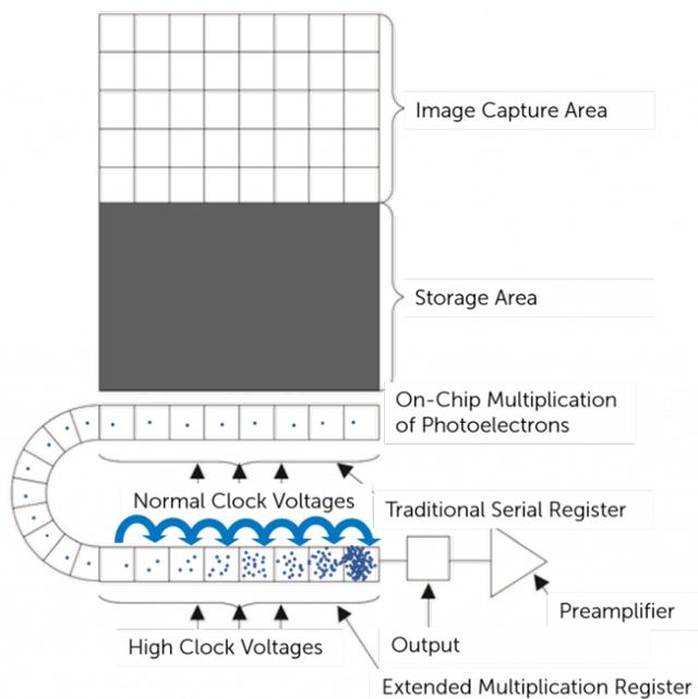
**Figure 2:** Schematic showing the architecture of an EMCCD sensor, with an image capture area and storage area for short frame times and an EM register with on-chip multiplication.
