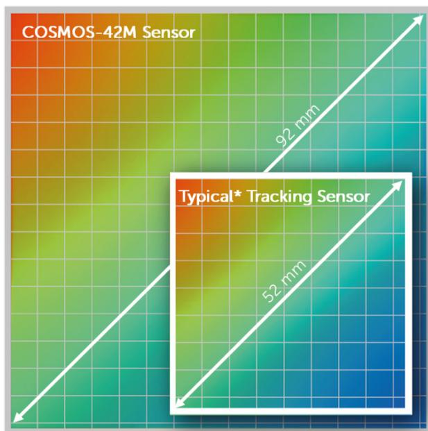
**Figure 5:** Graphical representation of the physical size of the COSMOS-42M (6496 x 6496) sensor versus a typical tracking sensor. \*Typical sensor based on a 9-micron pixel, 4096 x 4096 CCD sensor.
