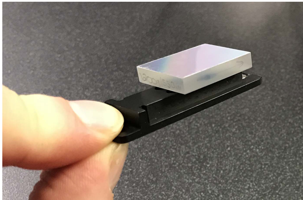
Figure C-7: Typical IsoPlane 81 Grating/Grating Carrier Assembly
