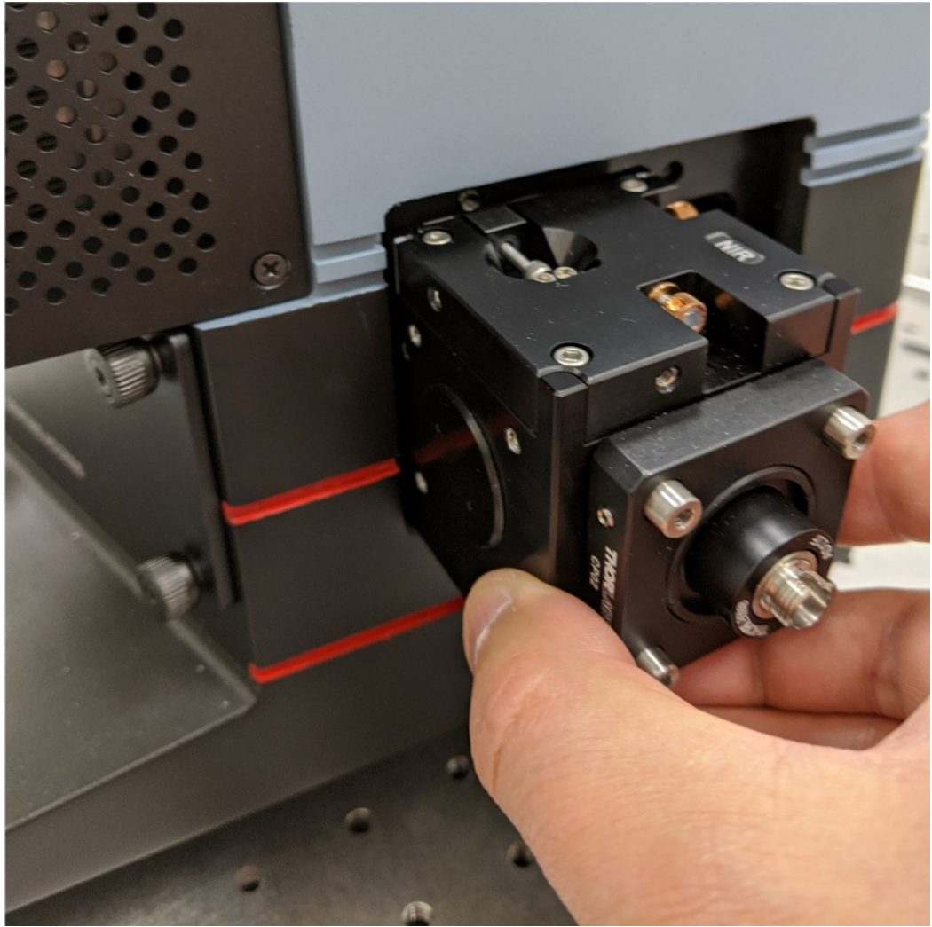
Figure 4-6: Installing the Focusing CUBE
