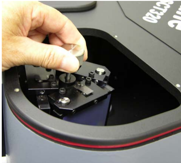
Figure 3-5: Lowering Turret into Turret Compartment
