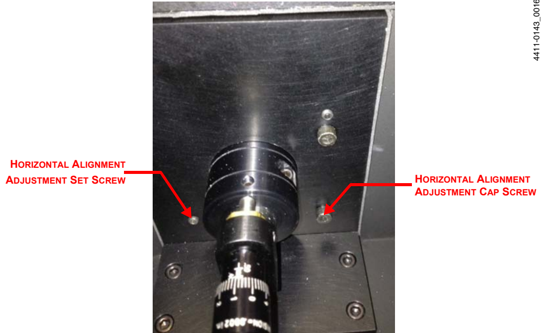
Figure 5-6: Horizontal Alignment Adjustment Screws
