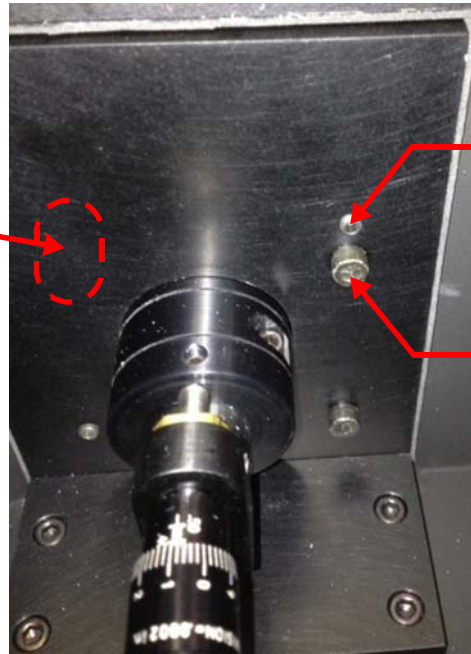
Figure 5-5: Vertical Alignment Adjustment Set Screws
