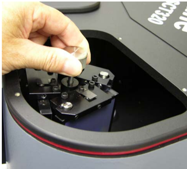
Figure 3-8: Removing the Grating Turret from the Grating Compartment
