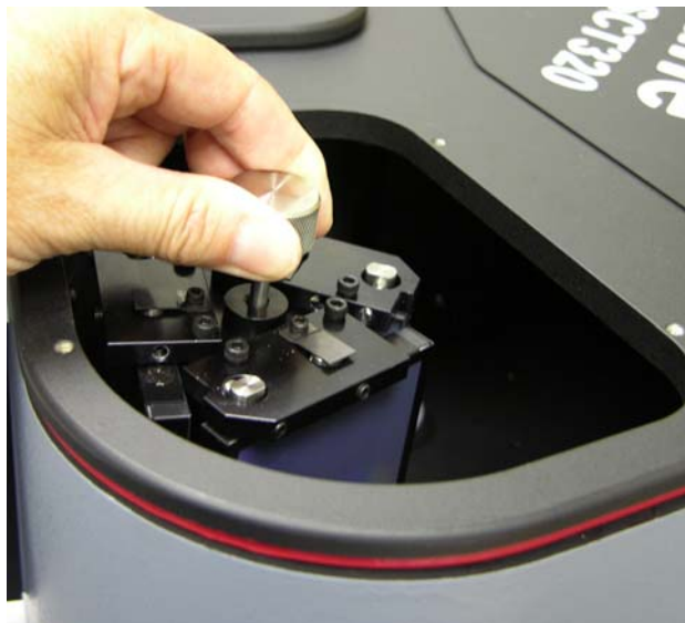
Figure 3-10: Removing the Grating Turret from the Grating Compartment
